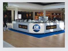
to optimize the use of its rental space. Made from pre-assembled units and equipped with casters, the islands provide the greatest possible flexibility for taking full advantage of the rental space in the mall. Illuminated ad space and interchangeable front panels display the DZ brand and the logos of the tenants.
