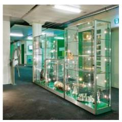
illuminated display cases for the various exhibits. They are easy to operate, strong and partially mobile. A mixture of standard and museum display cases was used. Some are attached to the walls, others serve as free—standing room dividers. The color of the bases and display case bottoms was chosen to match the original team colors of FCSG. For the lighting SYMA added flexible, easy-to-use low-voltage spots.
